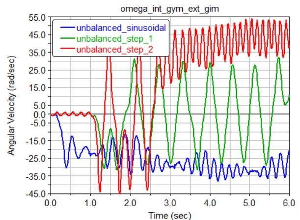
Fig. 7. Angular velocity in revolute joint between external end internal frames (unbalanced rotor).
