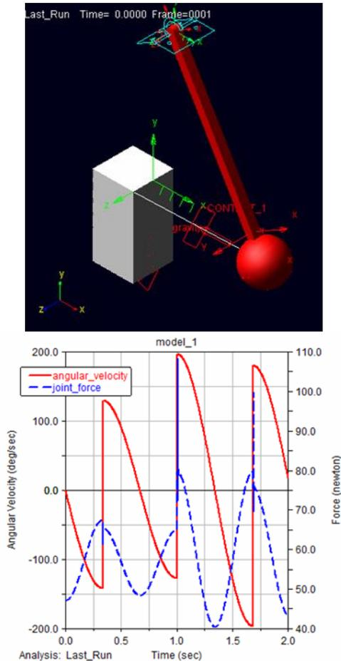
Fig. 2. Angular velocity and force variation with time in a revolute joint – impacting pendulum case.
