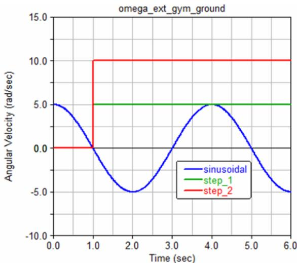
Fig. 5. Angular velocity imposed on external ring.
