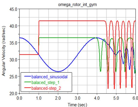
Fig. 10. Angular velocity in revolute joint between internal frame and rotor (balanced rotor).
