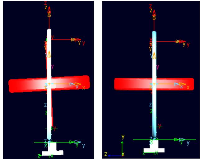
Fig. 6. Gimbals with dynamic unbalanced rotor a) and balanced rotor b).
