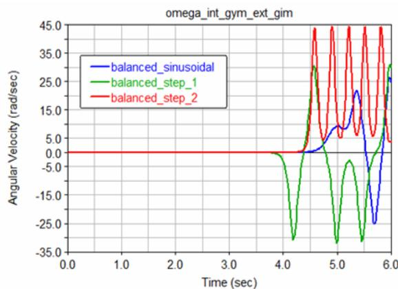
Fig. 9. Angular velocity in revolute joint between external end internal frames (balanced rotor).
