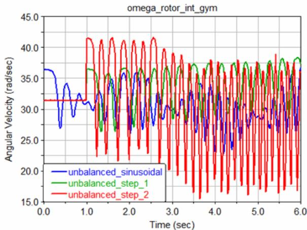
Fig. 8. Angular velocity in revolute joint between internal frame and rotor (unbalanced rotor).
